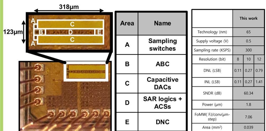
Figure 3. Die photo and measured result with different resolutions.
