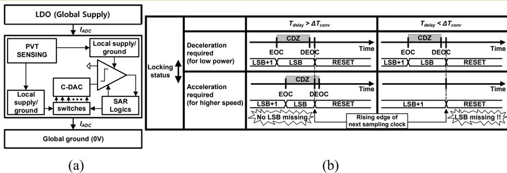
Figure 1. (a) The conceptual block diagram of proposed PVT compensation; (b) Criteria to prevent LSB missing in locking state
