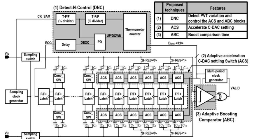
Figure 2. Block diagram of proposed SAR ADC.
